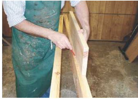
▲ Pic.2 The thickness of the boarding dictates the positions of the mortises...
